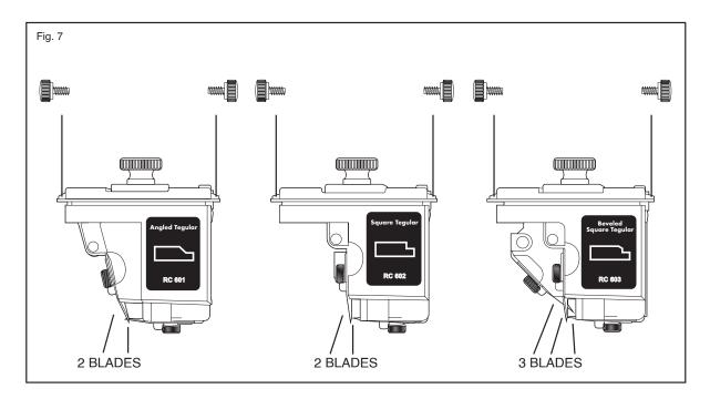
The profile blades are now installed. To remove and replace used blades, use the same procedure. Use the sharps container to dispose of used blades.
